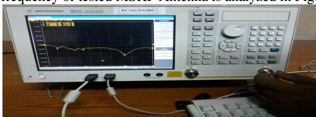
Figure.12. Testing of MSHP Antenna (By Setting the Start frequency, Stop frequency & Sample Points)
