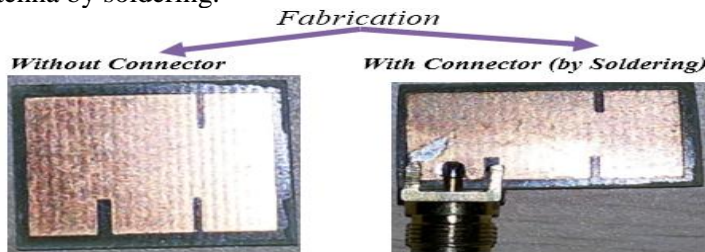
Figure.10.Fabrication of MSHP Antenna
